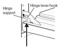
Lock engaged for door removal Figure 1
